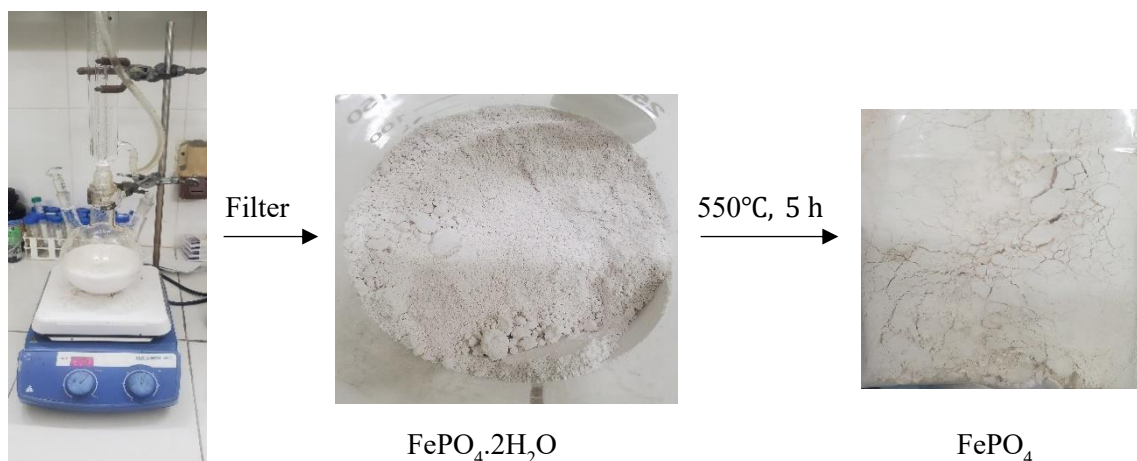
Figure 2.2. Experimental procedure for synthesizing \text{FePO}_4
