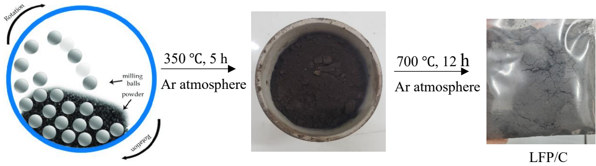
Figure 2.3. Experimental procedure for synthesizing LFP/C
